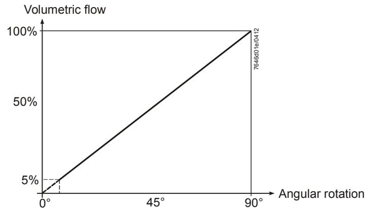
**Flow characteristic with rotation cylinder fully open (90°):**
